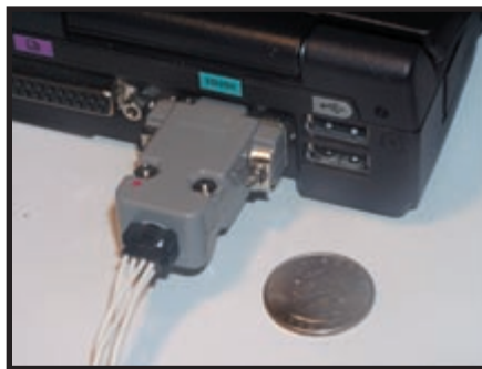
Photo 1 —My tiny AVR programmer plugs into a laptop's serial port. This diminutive device steals all of its operating power from the serial port's modem control lines.
