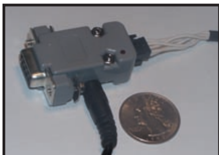
Photo 3 —External power is optional but useful for programming the programmer or using it without the serial port.
